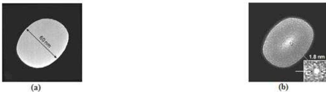
Figure 3: (a) Initial 61 nm pore on  $\text{Si}_3\text{N}_4$  (b) 1.8nm pore formed after sputtering with argon ions. [12]
